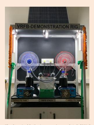
The Sustainable Environergy Research Lab (SERL) of Chemical Engineering Department, IIT Delhi has demonstrated working prototype of Vanadium Redox Flow Battery (VRFB). The vanadium redox flow battery can efficiently store and utilize renewable energy for a wide range of applications such as rural electrification, e-vehicle charging station, domestic and commercial power back-up etc. leading to zero carbon footprint.
